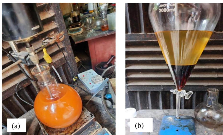
Figure 2. Oil in the stirrer during transesterification and Biodiesel/glycerol after transesterification: (a) During transesterification, (b) Biodiesel/glycerol after transesterification.
